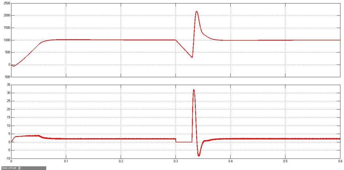
Fig.5 The speed and electric torque of PMSM without voltage gradual regulation
